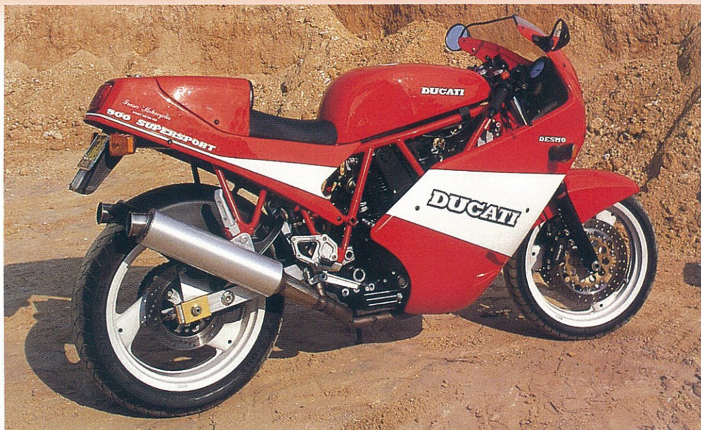
Below: Air cooled cylinders mount to 851 bottom end. Note frame and cantilever shock.
